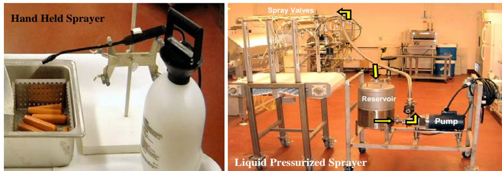
Figure 1. Equipment used for spraying electrolyzed water onto meat products. Handheld manual sprayer (left) and automated pressurized sprayer (right).
